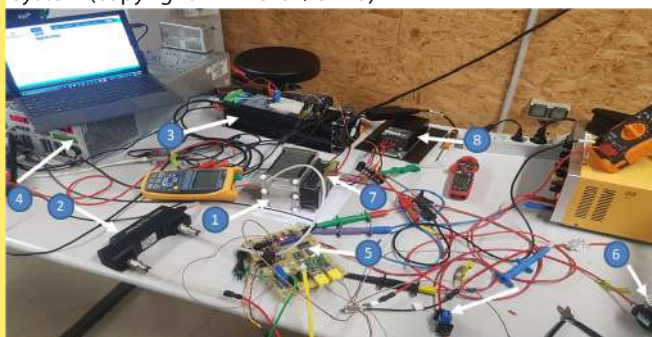
Experimental validation on an open-cathode 200W PEM fuel cell system (copyright FEMTO-ST/CNRS)
